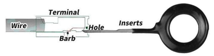
Step 2: Use the removal tool to push forward to unlock the barb and teminal
